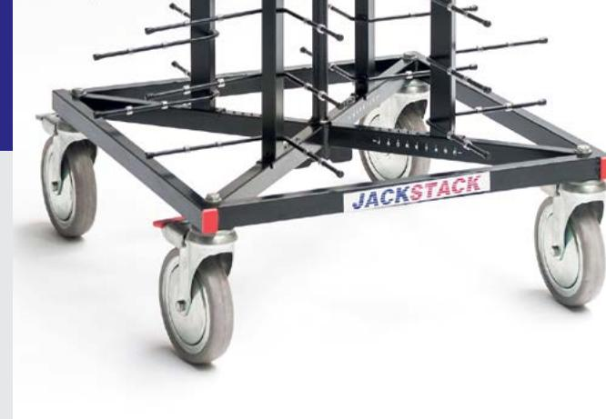
All mobile plate racks are equipped with 4 swiveling wheels (Ø 15cm/6") of which 2 with brake.
